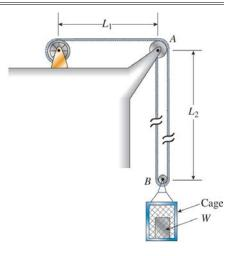
**2.2-9** An aluminum wire having a diameter d = 2 mm and length L = 3.8 m is subjected to a tensile load *P* (see figure). The aluminum has modulus of elasticity E = 75 GPa.
