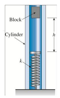
**Problem 2.8-10** A bumping post at the end of a track in a railway yard has a spring constant k = 8.0 MN/m (see figure). The maximum possible displacement d of the end of the striking plate is 450 mm.
